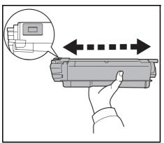
Take the new toner container out of the toner kit. Shake the new toner container at least 5 or 6 times as shown in the figure in order to distribute the toner evenly inside the container.
